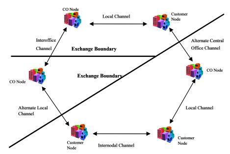
A customer configuration interface or company configuration interface may apply at each node. The rate element applies for capacity that originates or terminates at a node. Configuration interfaces provide for electrical (DS1, DS3, STS1, OC3c, OC12c) or optical (OC3 and OC12) channelization.
