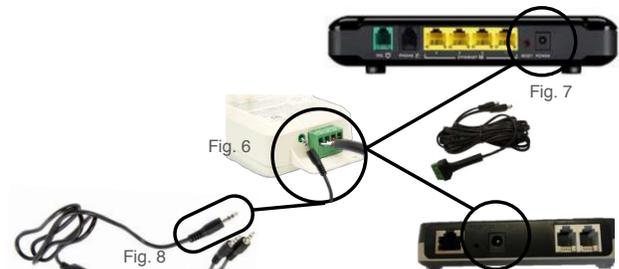
C. Connect "Y" Cable [Fig. 2] to the DCell BBU Input Port [Fig. 6] using the "Y" Cable Input Connector [Fig. 8]
